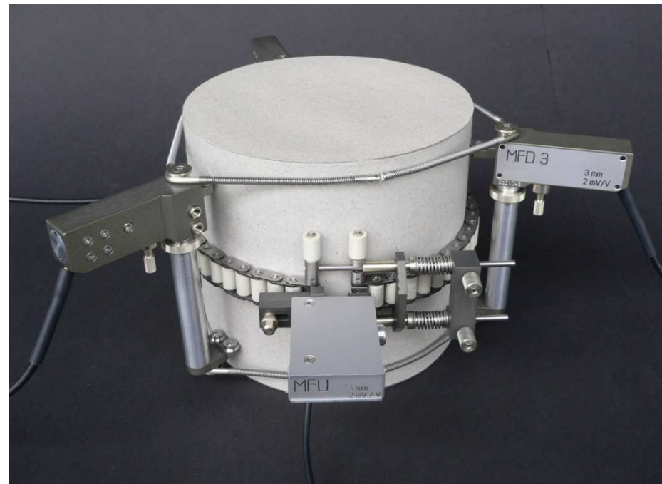
Picture 1: Extensometer system MFD 3 with MFU 4 for measuring circumferences Smallest initial gauge length of MFD 3 combination with MFU 4 = 60 mm
